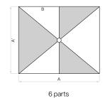
Loose cover max. 10 cm, concrete thickness min. 30 cm (pay attention to frost depth), Guarantee water drainage  $\,$
