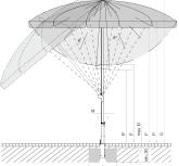
Loose cover max. 10 cm, concrete thickness min. 30 cm (pay attention to frost depth), Guarantee water drainage
