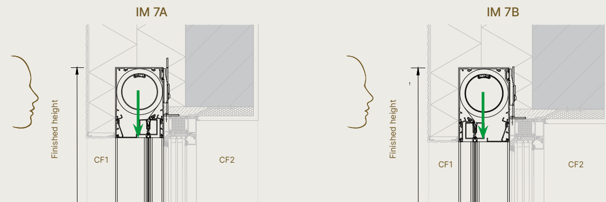
Medium - Drawing recessed plaster
